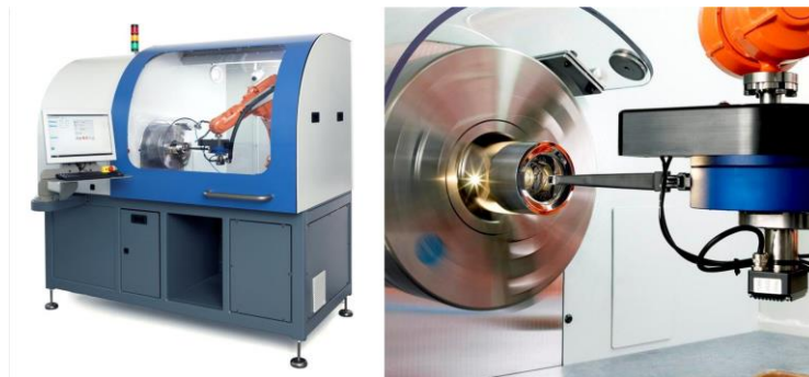
Figure 1; STRECON's Robot Assisted Polishing (RAP ® ) machine tool (left) and polishing module with oscillating tool motion close up (right) (Pilný et al. 2013).
