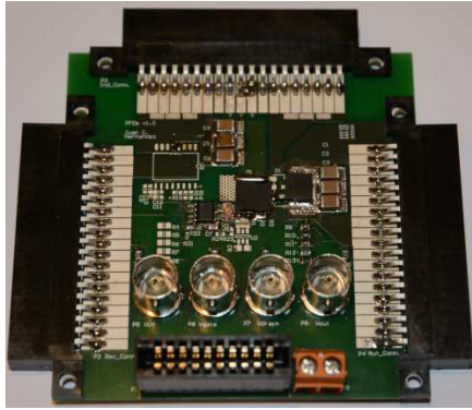
Fig. 14 Implemented modular PFC power stage
