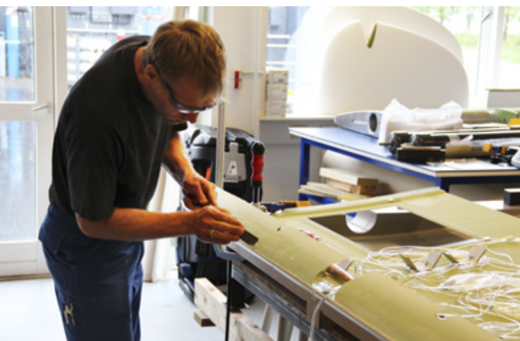
Fig. 2. Manufacturing the flap prototypes
