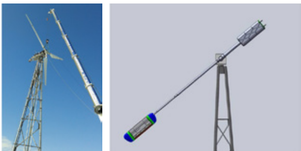
Fig. 4 and 5. The flap system will be tested on a blade 2m x1m blade section mounted on a 10m long boom replacing the standard rotor on the 100kW Tellus turbine at Risø Campus. In this way almost similar working conditions as a full scale turbine are obtained.
