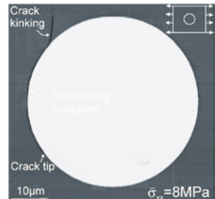
Fig. 3. Debonding and crack kinking observed during transverse tensile testing in scanning electron microscope.
