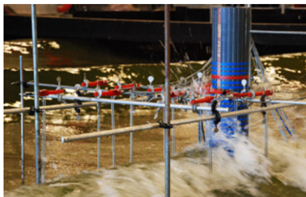
Fig. 2. Model test at DHI with a monopile exposed to breaking waves.
