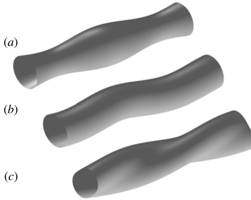
FIGURE 1. Main vortex cavity oscillation modes reproduced from Bosschers (2008). With (a) monopole breathing n = 0 mode, (b) dipole serpentine n = 1 centreline displacement mode and (c) quadrupole helical n = 2 mode.
