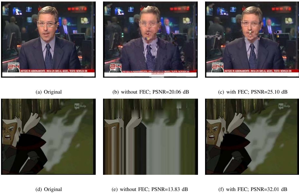
Figure 4 Comparison of visual effects on decoded frames for the videos 'News' and 'Cartoon' at 2 Mbps with and without FEC technique. The overhead is equal to 20%, and PLR is equal to 9%.
