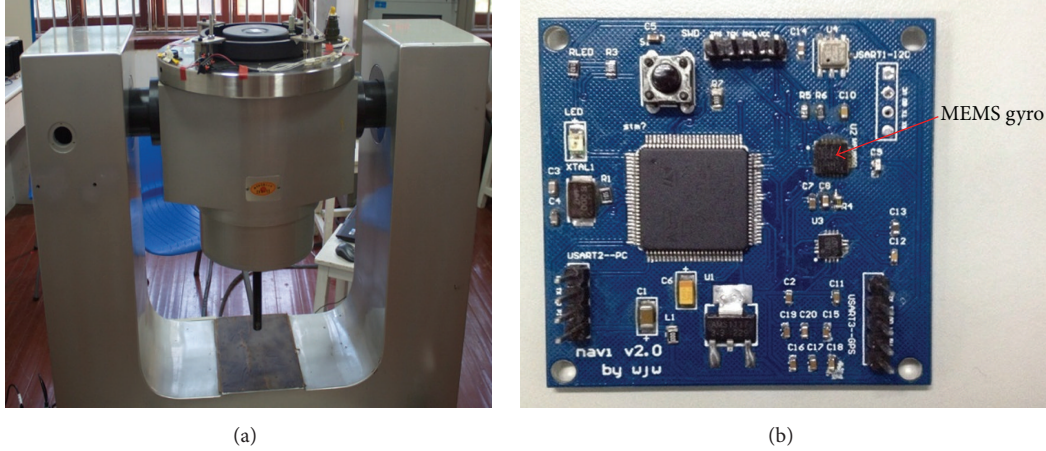
FIGURE 2: FOG and MEMS gyros: (a) FOG on turntable and (b) MEMS gyro.
