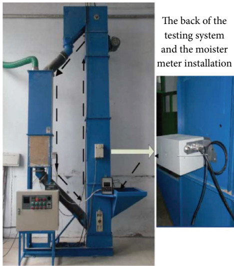
FIGURE 10: Self-designed grain moisture comprehensive test system.
