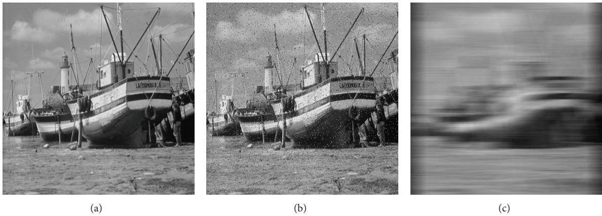
FIGURE 18: (a) Image of Boat; (b) noisy image with “salt and paper” noise with noise density of 0.03; (c) blurred noisy image degraded by a uniform horizontal linear motion of length 85.
