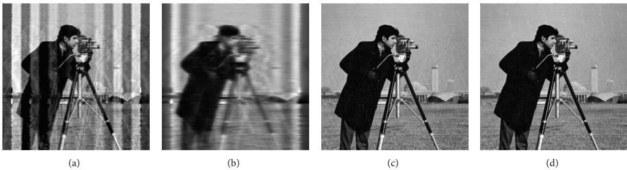
FIGURE 21: Restoration of Cameraman with (a) WF, (b) LR algorithm, (c) Haar basis ( \kappa = 10 ), and (d) Fourier basis ( \kappa = 40 ).
