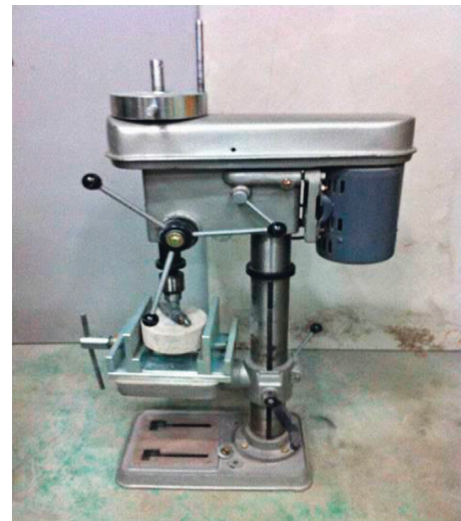
FIGURE 6: Abrasion test setup.
