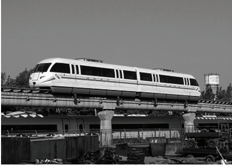
FIGURE 1: CMS04 maglev vehicle in National mid-low speed maglev experiment field of Tangshan city.
