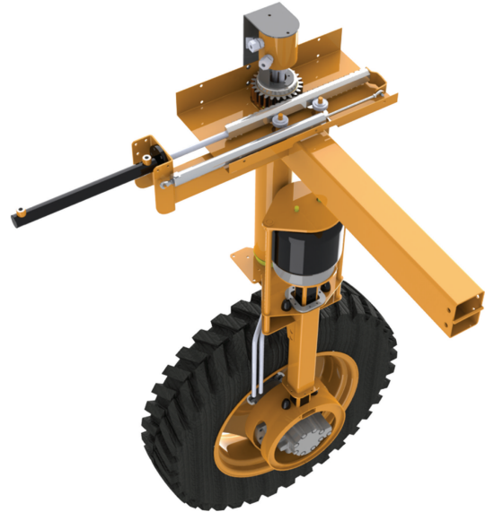
FIGURE 3: Representation of a wheel module of the robot steering system.
