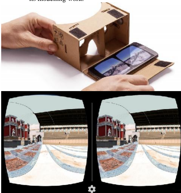
Figure 13. The VR application, allowing to explore full dome views of 3D model wearing Google Cardboard
