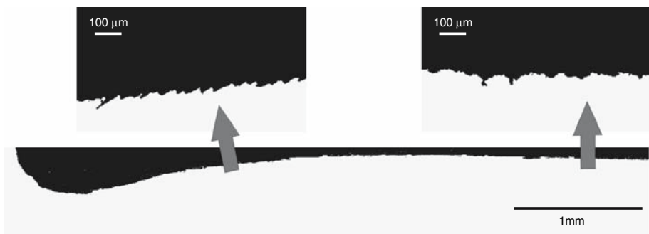
Fig. 6 Macroscopic ( bottom , front shown from edge to centre-line of sample) and microscopic crack front geometry top at very low front speeds (<1 nm/s) derived from optical micrographs. Crack moves from the bottom upwards, delaminated areas are white. Residual stress state likely causes macroscopic crack shape (compare Fig. 7). Different microscopic crack front geometry exists at different positions along the crack front. Top left: microscopic front geometry left of centre at position indicated by arrow. Top right: microscopic front geometry along the centre line
