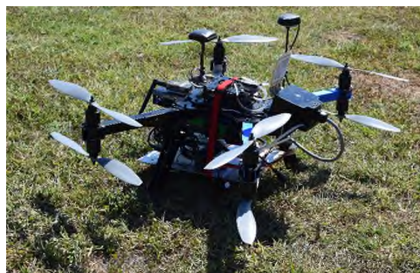
Figure 6. Setup for second campaign. IMST radar is slightly pitched down.
