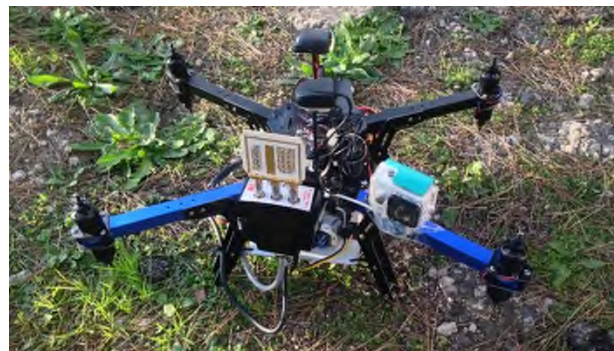
Figure 4. Setup for first campaign. IMST radar is mounted in forward-looking position.
