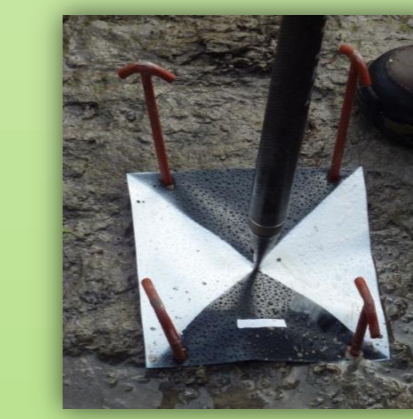
Figure 5. An artificial ground control point (GCP)
