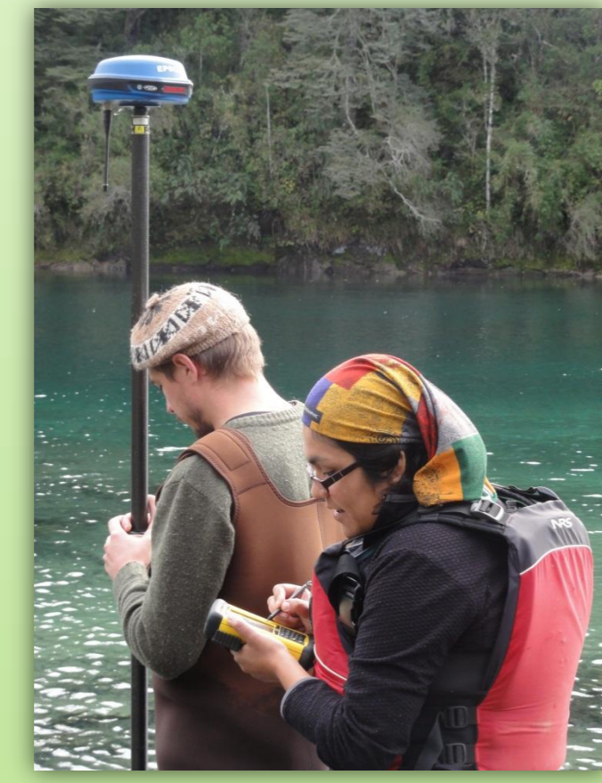
Figure 1. Surveying fluvial topography using a dGPS
