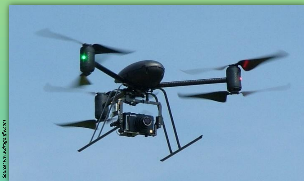
Figure 2. The Draganflyer X6 – an unmanned aerial system
