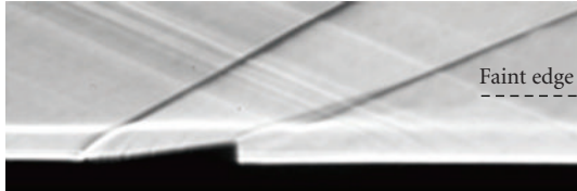
FIGURE 6: The experimental schlieren by Babinsky et al. [7].
