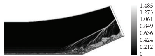
FIGURE 4: The digital schlieren at central plane.
