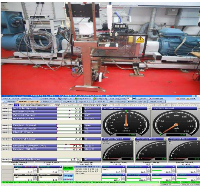
Figure 1 – Testing rig used for current study showing the generator type dynamometer (top) as well as the software interface (bottom).
