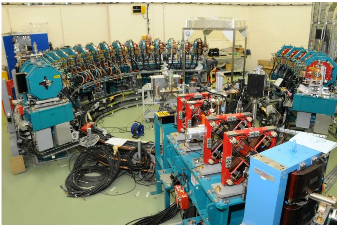
Figure 7: EMMA as of the beginning of 2010. This shows the end of the injection line and the 4 (out of 7) ring girders in place at the time.
