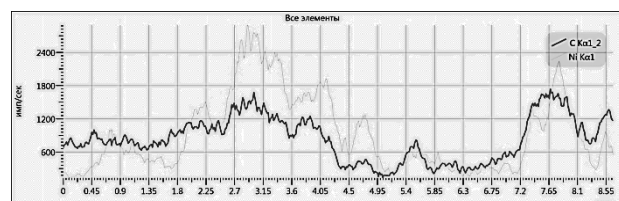
Fig. 3 – Carbon (black line) and nickel (grey line) profiles according to energy dispersive analysis data
