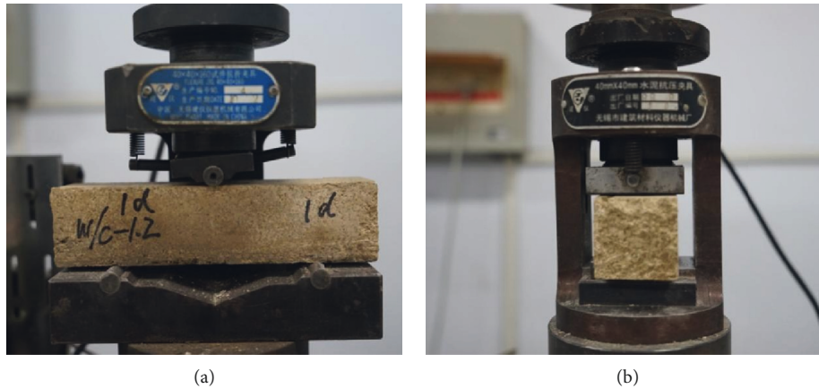
FIGURE 4: (a) Flexural strength test. (b) Compressive strength test.
