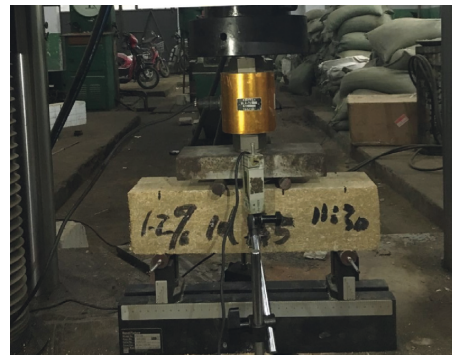
FIGURE 5: Flexural toughness test.
