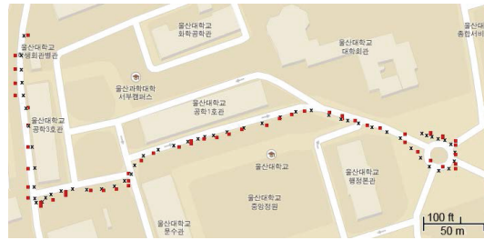
FIGURE 6: Result of the proposed method, where the red blocks are real GPS data received from the receiver and the black crosses are the results of the proposed method.
