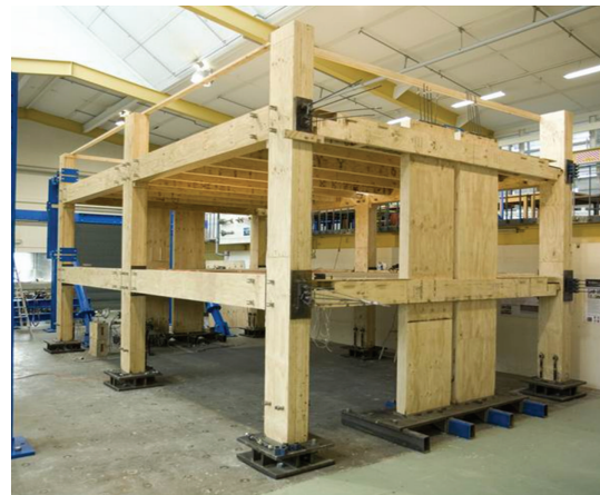
FIGURE 2: Experimental posttensioned timber building in the laboratory of the University of Canterbury with TCC floors.
