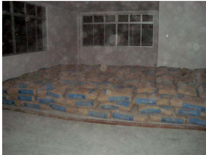
Figure 2: Cement bags used as the test load
