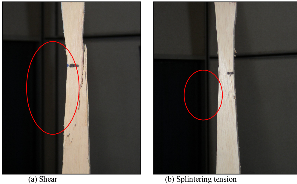
Figure 4: Failure found in tensile test rubberwood LVL
