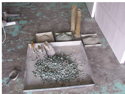
Figure 4. Materials ready to be mixed
