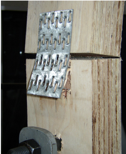
Fig. 2 Teeth withdrawal failure in rubberwood LVL
