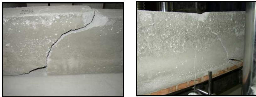
Figure 6 Crack Pattern for Control and Composite Beam 1
