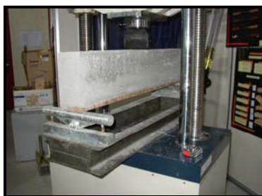
Figure 2 Typical Setup of Flexural Strength Test
