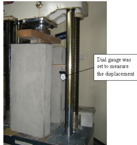
Figure 3. Setting up of TLCC Push-Out Test
