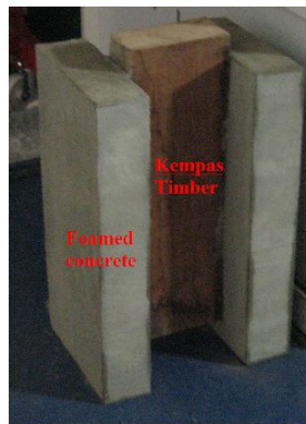
Figure 3: TLCC Push-out test specimen
