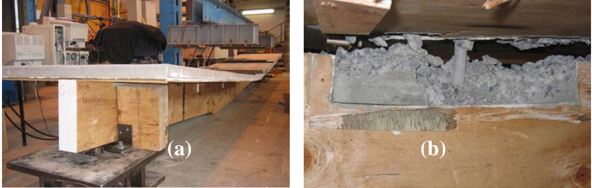
Figure 5: Different types of failure mechanisms detected in the composite beams: (a) fracture in tension of LVL; (b) failure for concrete shear and crushing in 300 mm rectangular notched connection
