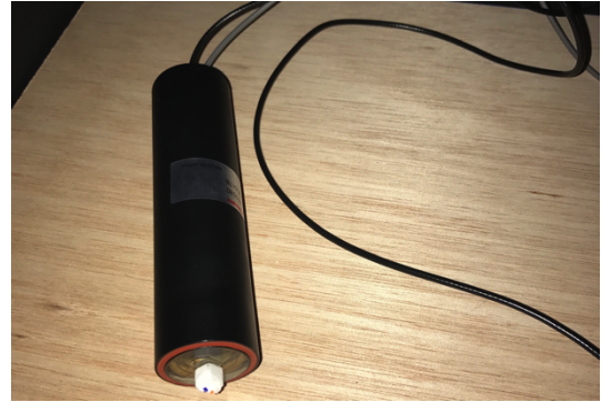
Fig. 13: A 6 mm x 6 mm stilbene crystal coupled to a Hamamatsu H10580 PMT assembly.
