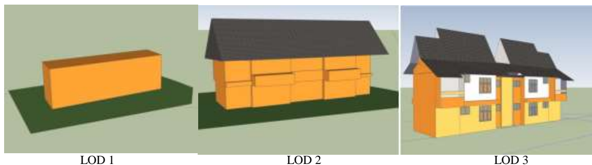
Figure 9. Resulted model in LOD 1, LOD 2, and LOD 3.
