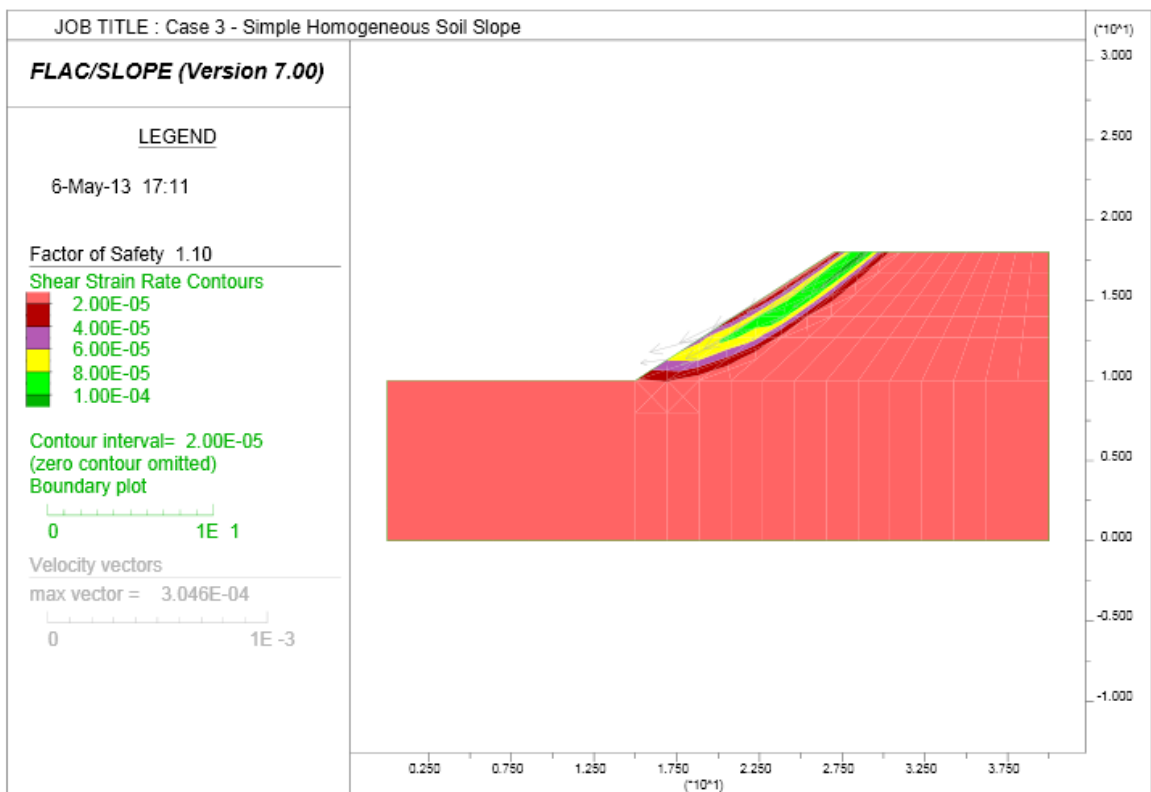
Figure 13 FLAC/Slope Critical Slip Surface for Case 3 - Simple Homogeneous Soil Slope
