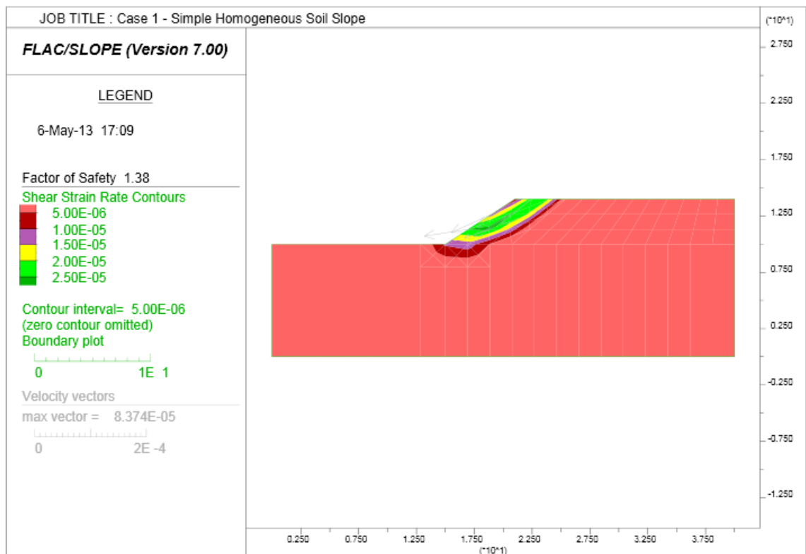
Figure 11 FLAC/Slope Critical Slip Surface for Case 1 - Simple Homogeneous Soil Slope
