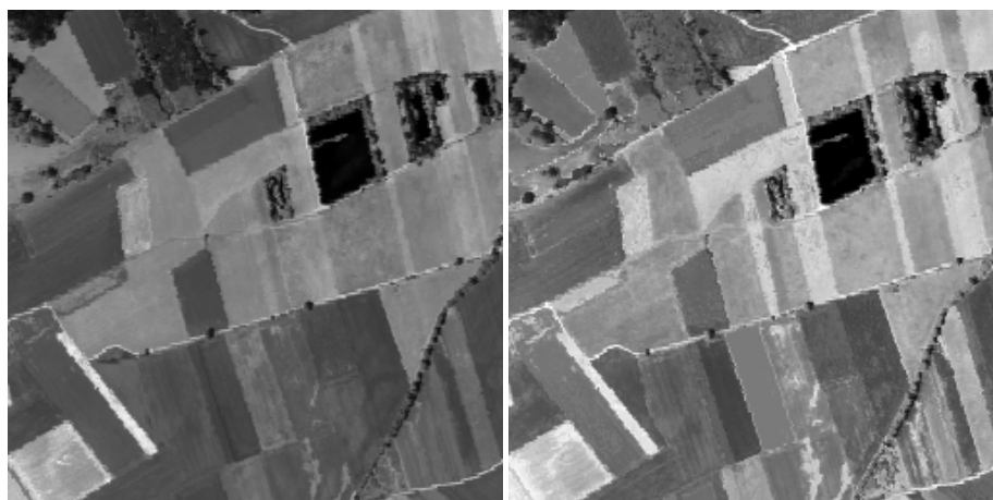
(e) Original 256 \times 256 hyperspectral image, channel 80. (f) Restored 256 \times 256 hyperspectral image, channel 80.
