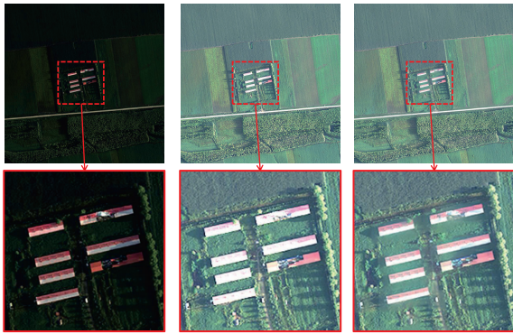
Figure 6. An illustration of our proposed structure transferring algorithm: (Left) the original image suffering from underexposure; (Middle) the adjusted result by exposure compensation via Photoshop ; (Right) the structure-transferring image, which not only presents the similar appearance with the adjusted image but also preserves the local structures of the original image.
