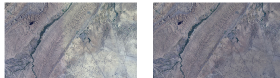
Figure 1. An example illustrating that blending can't obviously eliminate the tonal difference alone. The left mosaicked image was obtained directly by a multi-band blending technique. The right mosaicked image was generated by our proposed tonal correction followed by a multi-band blending technique.
