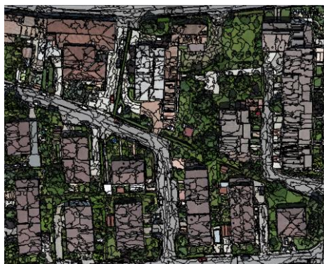
Figure. 7 urban features multi-scale Segmentation of Ortho photo made from taken images from UAV
