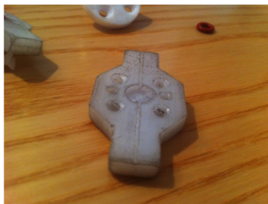
(a) Base layer: the groove and the inner tank are clearly visible.
