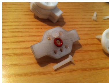
(b) Middle layer: silicon o-ring and nylon screws are fixed to it..
