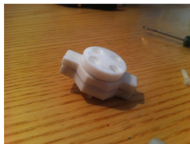
(d) The 3-layer holder assembled with nylon screws.
