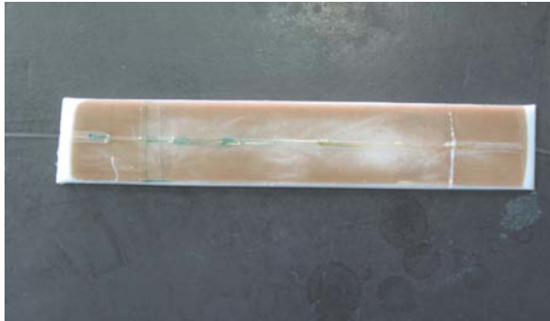
Figure 3.3: FBG bonded on a Teflon sample.
