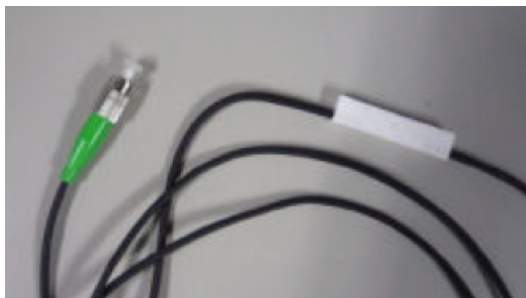
Figure 2.1: FBG sensor packaged with a ceramic material.
