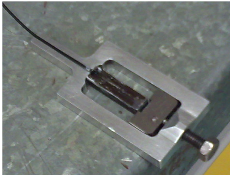
Figure 4.2: Picture of the FBG magnetic sensor: the black block is a magnetostrictive rod (Terfenol-D) on which is bonded a bare FBG. The sensor is placed in a pre-stress holder.
