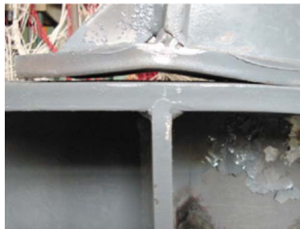
Figure 2.37: Moment-rotation curve and failure mode for EPC-5
