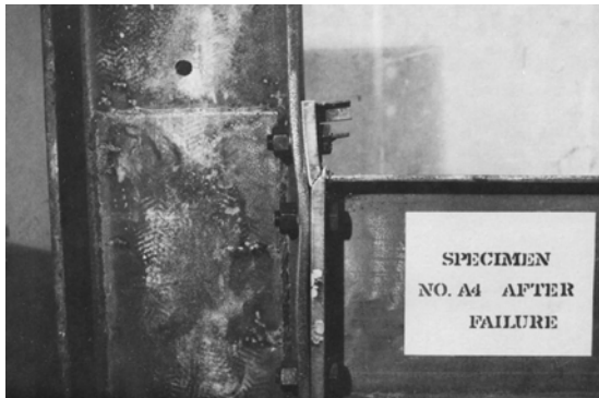
Figure 2.7: Beam load versus beam tip displacement curve and failure mode for A-4
