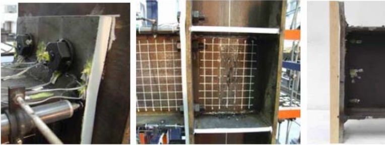
Figure 2.17: End-plate failure, column web panel and end-plate deformation for J-1.3
