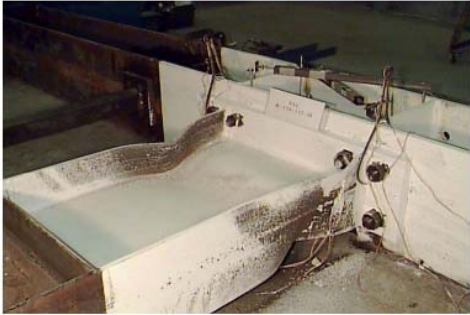
Figure 2.10: a) Moment rotation curve and b) failure mode for 4E-1.25-1.5-24
