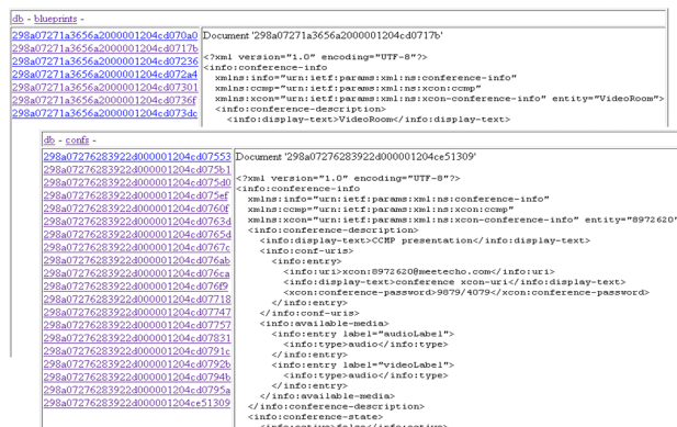
Figure 2.5: An image of the Xindice native XML database used in the prototype
