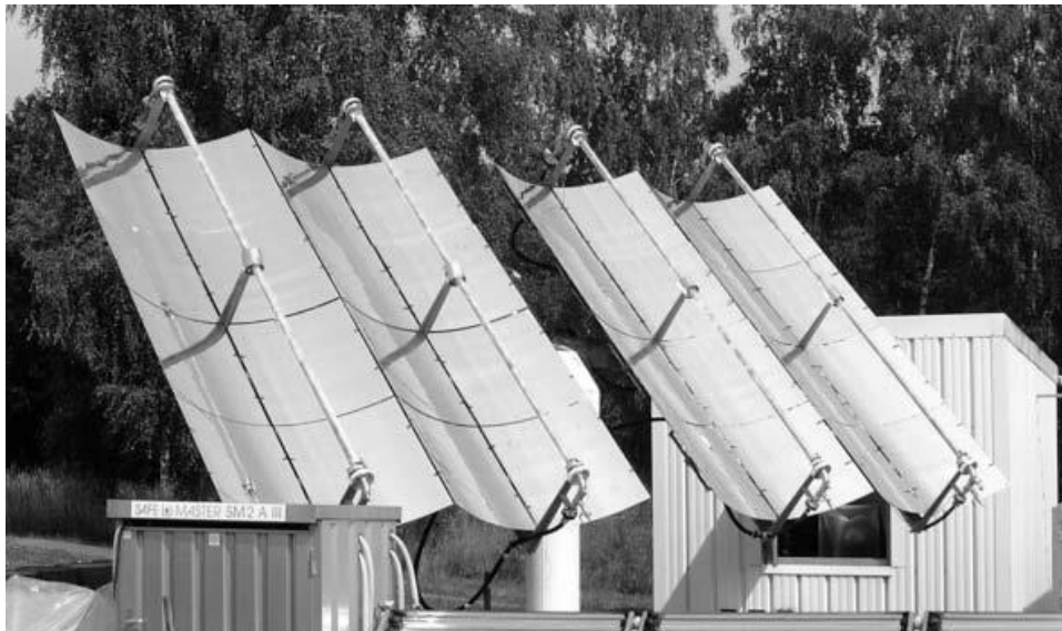
Fig. 12 PTCs reactors during the photooxygenation of citronello [14] .
