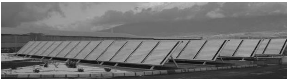
Fig. 14 CPC-solar reactors for the treatment of contaminated waters in southern Spain in El Ejido in the province of Almeria (Albaida S.A).
