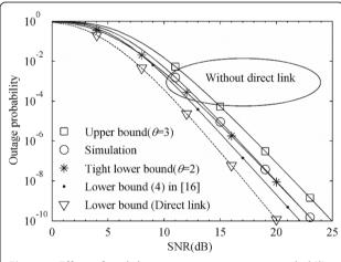
Figure 4 Effect of path loss exponent on outage probability for TWOR-AFNC systems under symmetric channels (K = 6).
