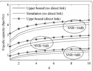
**Figure 2** Comparison of tight upper bound of ergodic capacity versus number of relays between TWOR-AFNC-Dir and TWOR-AFNC-Nodir (K = 10, p = 3,  $d_{1k} = 0.5$ ).
