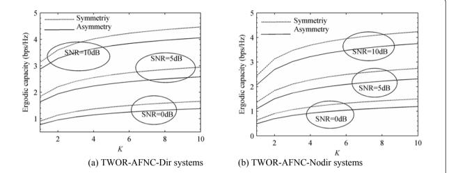
Figure 3 Comparison of tight upper bound of ergodic capacity versus number of relays between symmetric channels and asymmetric channels  $d_{1k} = 0.3$  for TWOR-AFNC-Dir and TWOR-AFNC-Nodir, respectively (K = 10, p = 3). (a) TWOR-AFNC-Dir systems; (b) TWOR-AFNC-Nodir systems.
