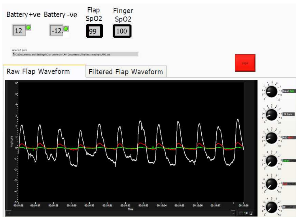
Figure 8.7: Front panel utilized for observing real-time flap PPG signals with adjustable gain and offset.
