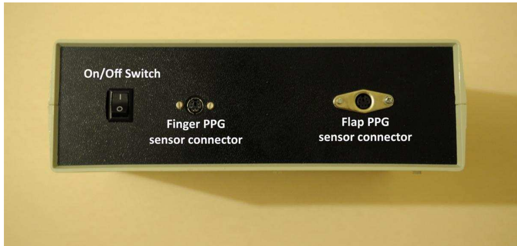
Figure 7.15: Front panel of the instrument case with the finger and flap channel sockets and the on and off power switch.
