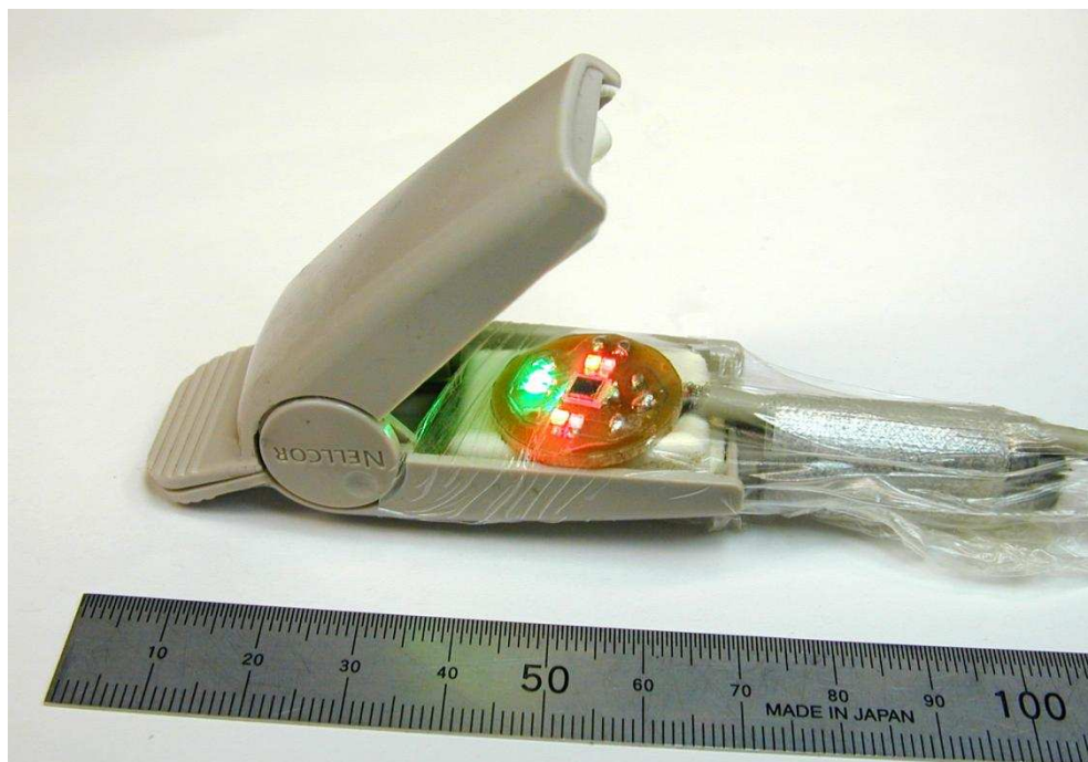
Figure 6.12: Photograph of the developed finger PPG sensor fixed into the commercial finger clip and covered with adhesive transparent film dressing with the LEDs switched on.
