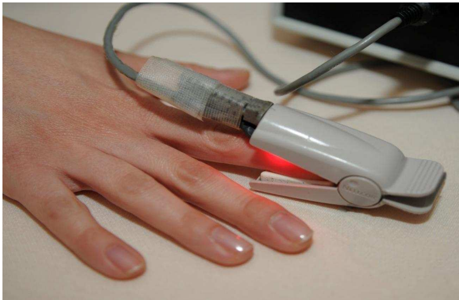
Figure 6.13: Photograph showing the finger PPG sensor on a volunteers' index finger for evaluation.
