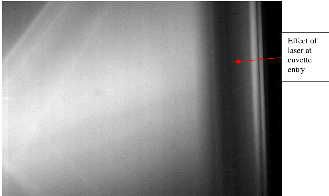
Figure 6.4 Mean laser profile at 10 kHz, 1mJ/pulse laser power.
