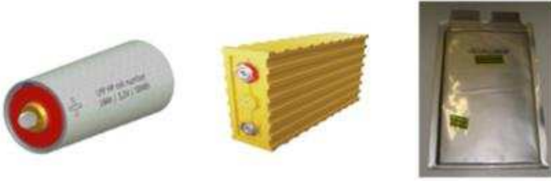
Figure 3: Cell designs (Cylindrical, Prismatic and Pouch) [4]
