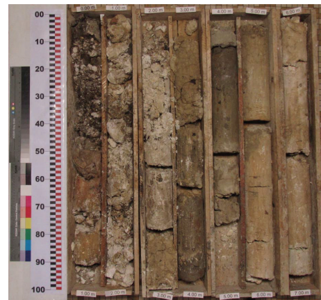
FIGURE 3: Soil samples obtained from the coring S1 on the crest of the embankment.
