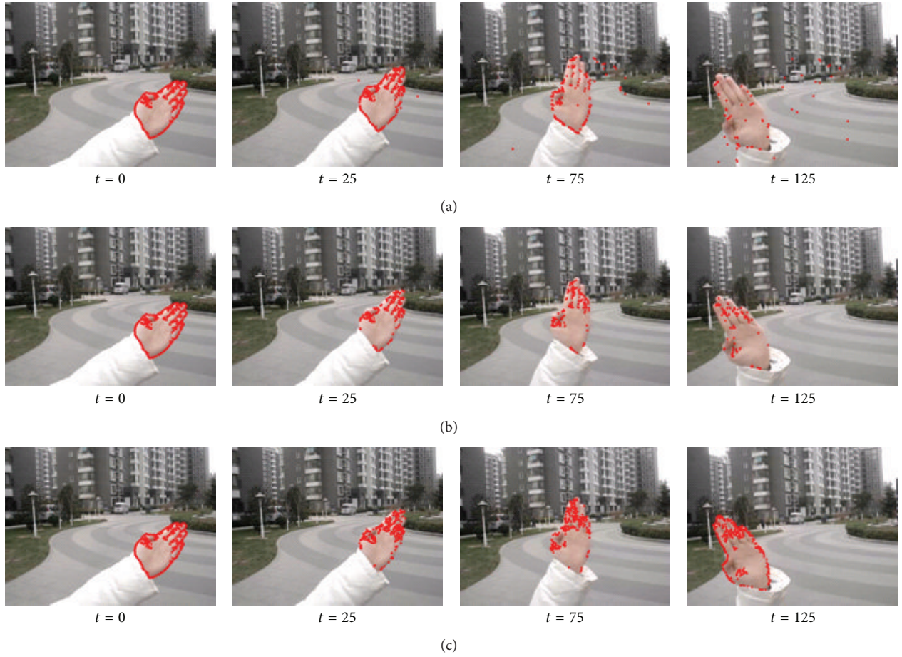
FIGURE 3: (a) Some points are out of hand range via optical flow at t = 75, 125 . (b) The degeneracy problem occurs (the number of points is drastically reduced at time t = 125 ). (c) Results by our method.
