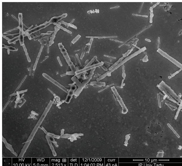
FIGURE 1: SEM image of the SCNRs, magnified 2513x.
