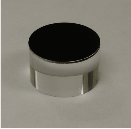
FIGURE 3: A dielectric resonator with carbon nanotubes deposited on the end surfaces.
