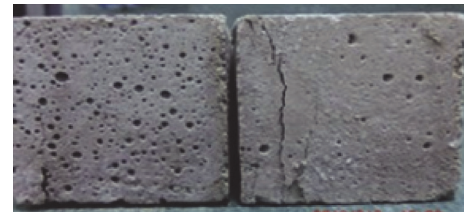
FIGURE 4: Mortar mixed with rubber particles compressive failure mode.
