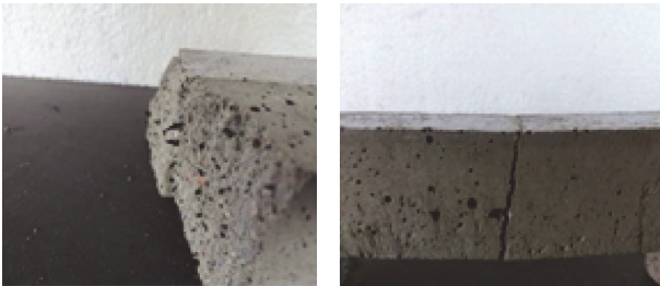
FIGURE 7: Mortar mixed with rubber particles flexural failure mode.
